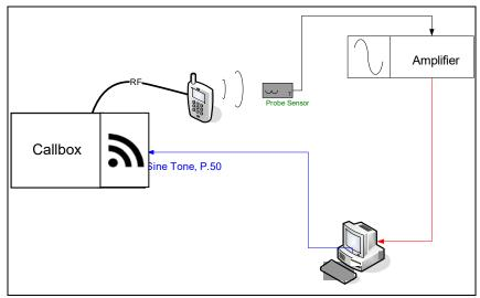
Figure 4-2 T-Coil Test Setup
