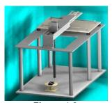
**Figure 4-3** RF Near-Field Scanner
