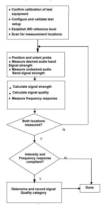
Figure 4-14 C63.19 T-Coil Signal Test Process
