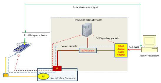
Figure 5-1 Test Setup for VoLTE over IMS T-Coil Measurements
