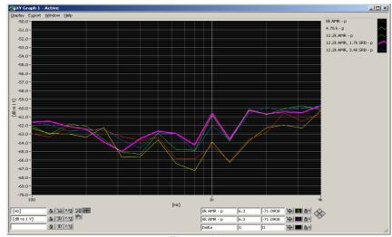
Figure 8-3 **UMTS Audio Band Magnetic Noise**
