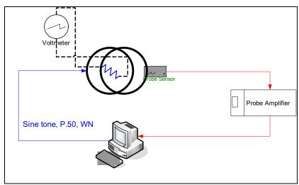
Figure 4-1 Validation Setup with Helmholtz Coil
