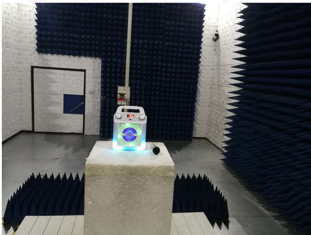
RADIATED EMISSION TEST SETUP ABOVE 1GHZ
