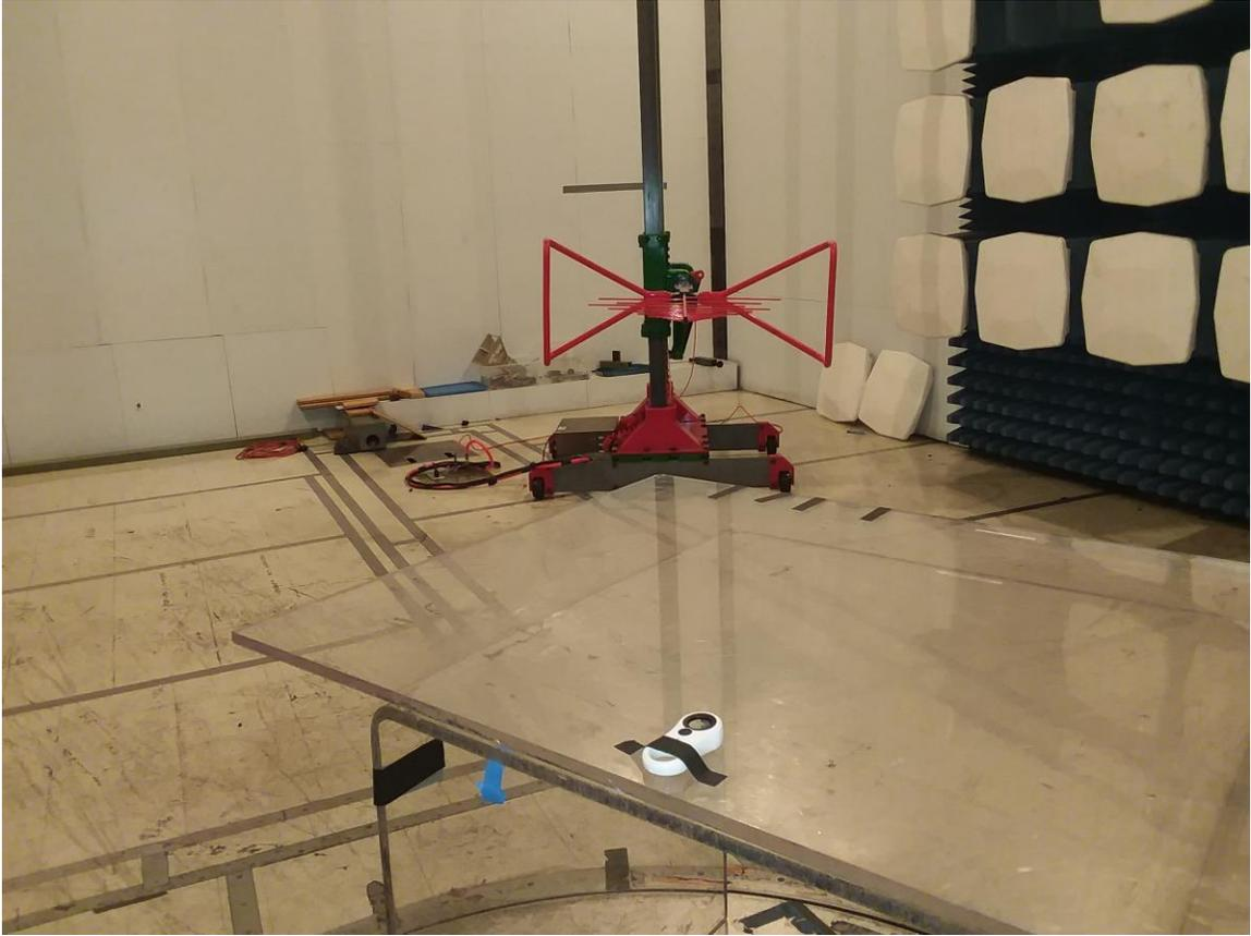
**Photograph 2. Radiated Spurious Emissions, 30-1000 MHz, Test Setup**
