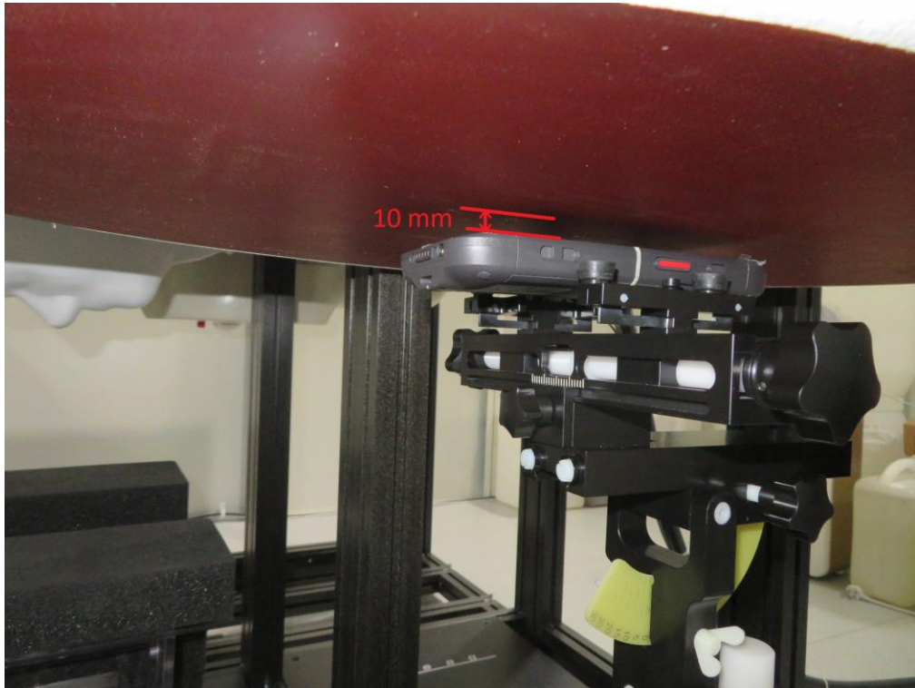
Description: Body Front with earphone with 10mm gap
