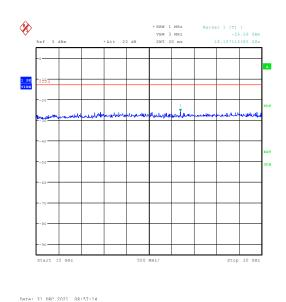
**Channel 9538: 30MHz –1GHz** Spurious emission limit –13dBm.
