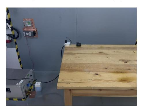
Set-up for Radiated Emission (RE), Below 1GHz
