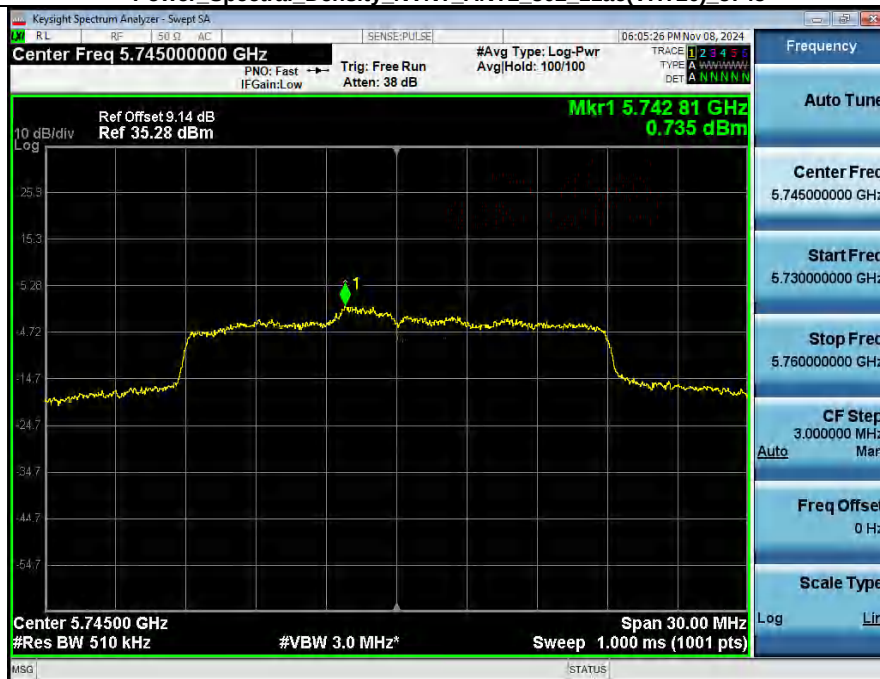
Power Spectral Density NVNT_ANT2_802_11ac(VHT20)_5745
