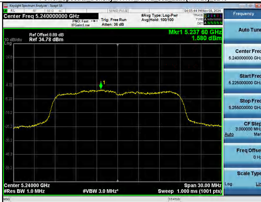
Power Spectral Density NVNT ANT2_802_11ac(VHT20)_5240
