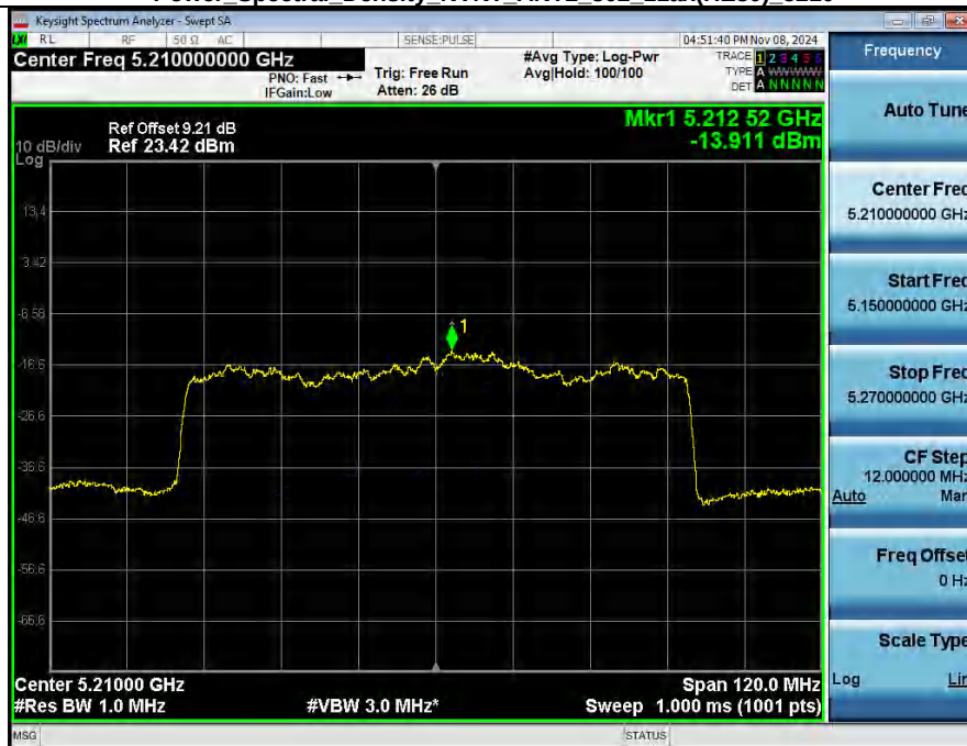
Power Spectral Density NVNT ANT2 802 11ax(HE80) 5210
