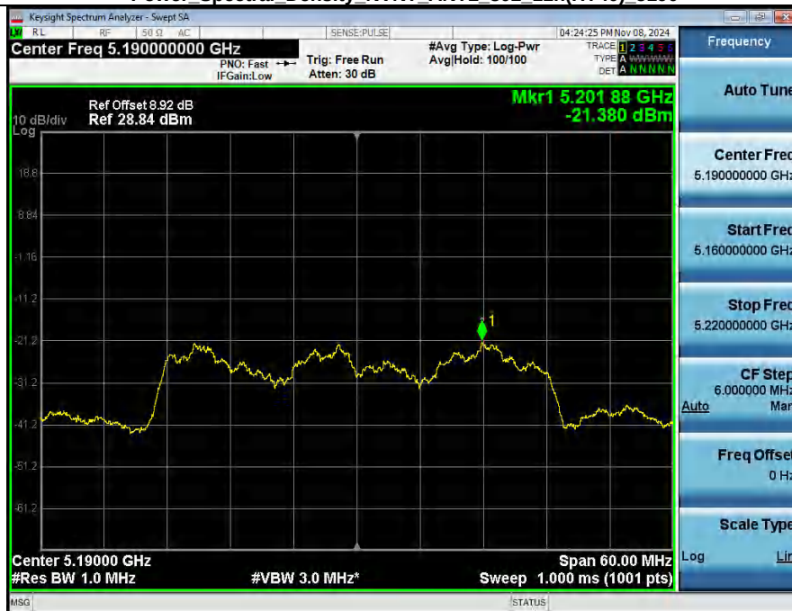
Power Spectral Density NVNT_ANT2_802_11n(HT40)_5190
