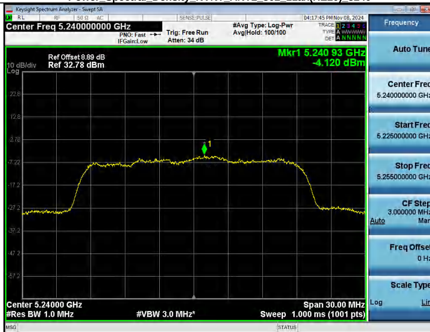
Power Spectral Density NVNT ANT2 802 11ax(HE20) 5240
