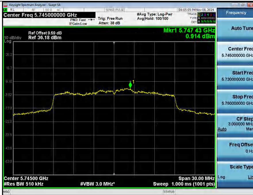
Power Spectral Density NVNT_ANT2_802_11ac(VHT20)_5745
