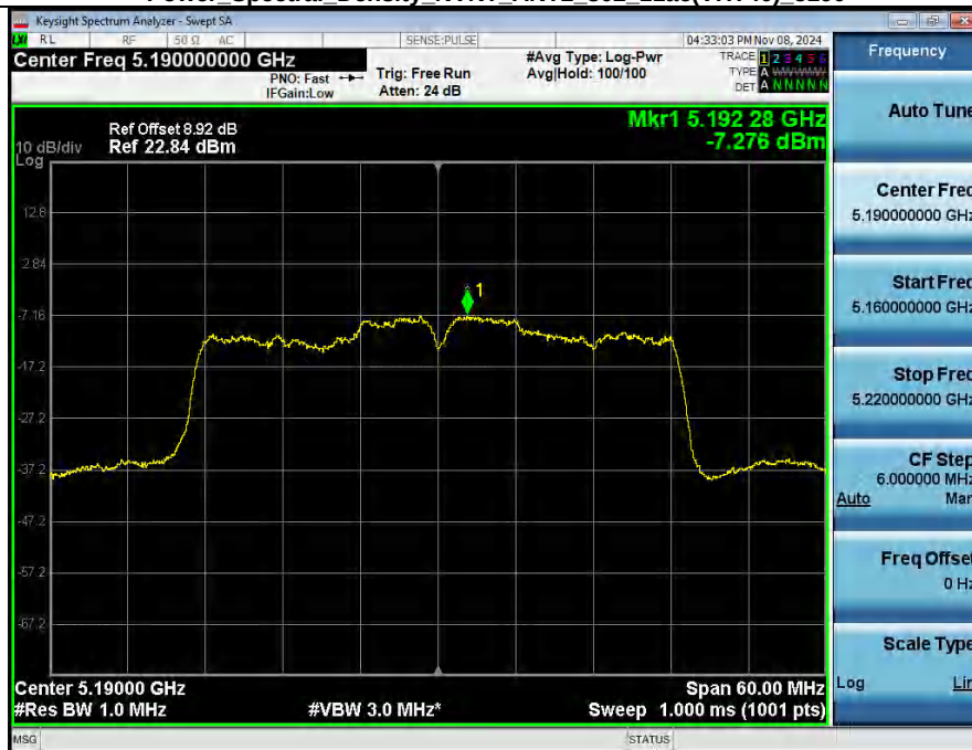
Power Spectral Density NVNT_ANT2_802_11ac(VHT40)_5190
