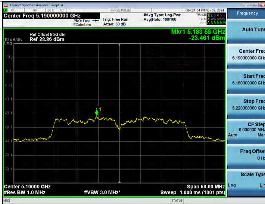
Power Spectral Density NVNT_ANT2_802_11n(HT40)_5190
