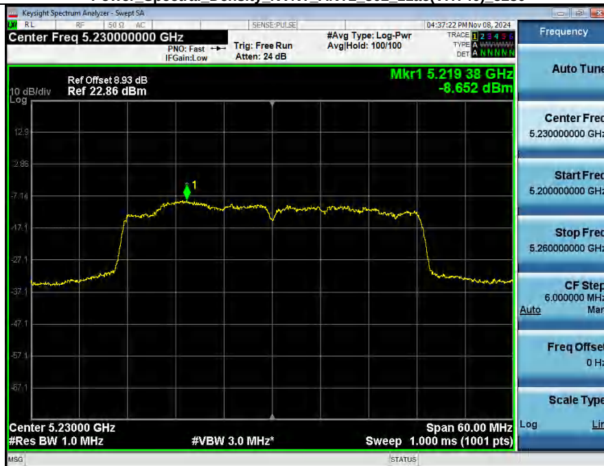
Power Spectral Density NVNT ANT2 802_11ac(VHT40) 5230
