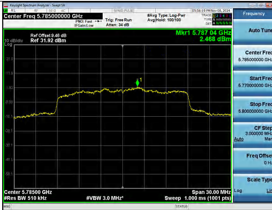
Power Spectral Density NVNT_ANT2_802_11n(HT20)_5785
