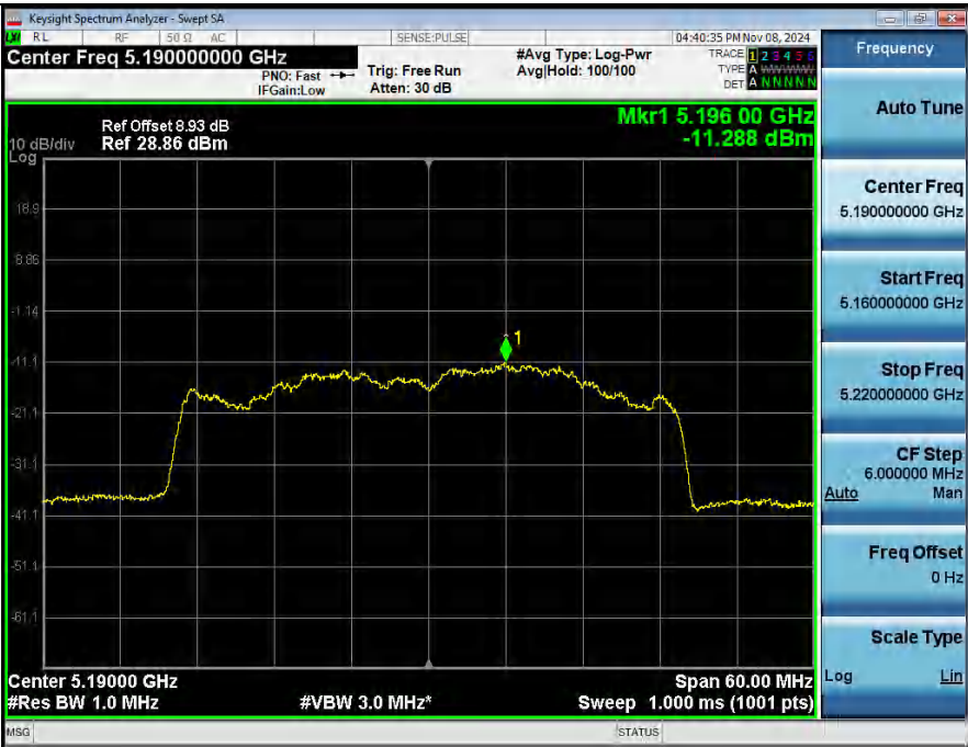
Power Spectral Density NVNT ANT2 802_11ax(HE40) 5190
