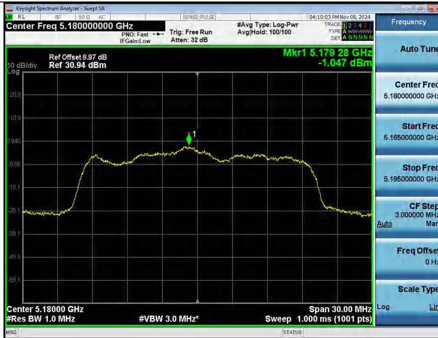
Power Spectral Density NVNT ANT2 802_11ax(HE20) 5180
