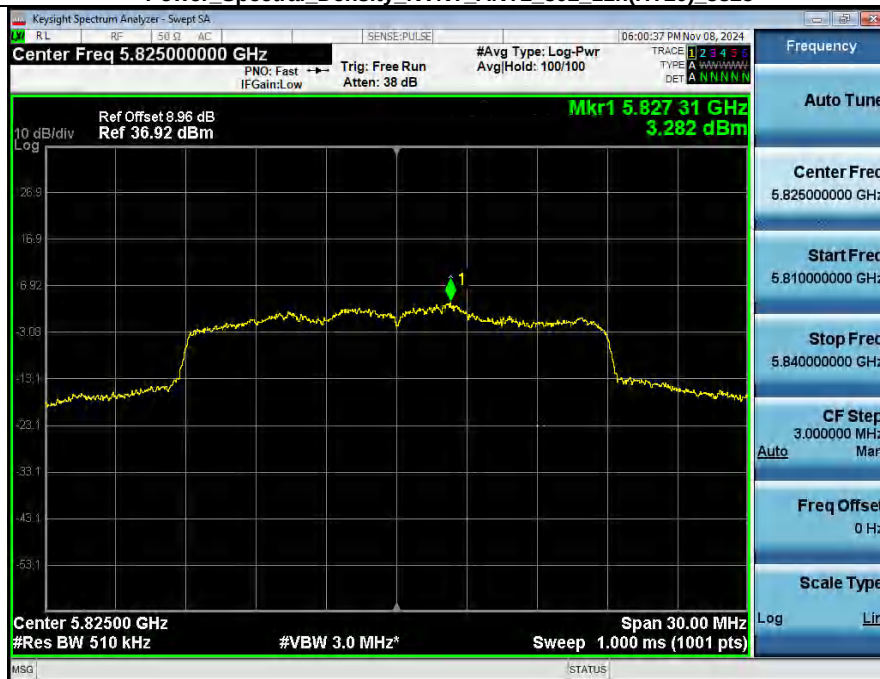
Power Spectral Density NVNT_ANT2_802_11n(HT20)_5825
