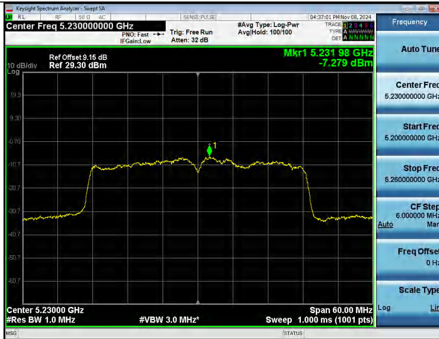
Power Spectral Density NVNT ANT2 802_11ac(VHT40) 5230
