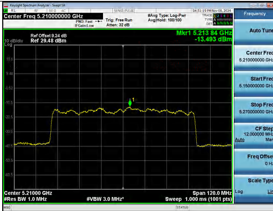
Power Spectral Density NVNT ANT2 802 11ax(HE80) 5210
