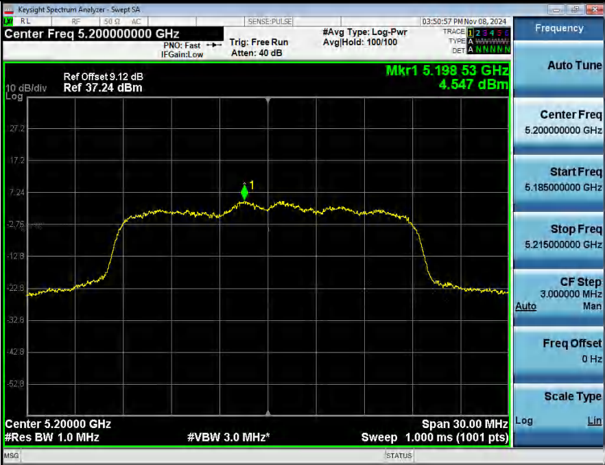
Power Spectral Density NVNT_ANT2_802_11n(HT20)_5200
