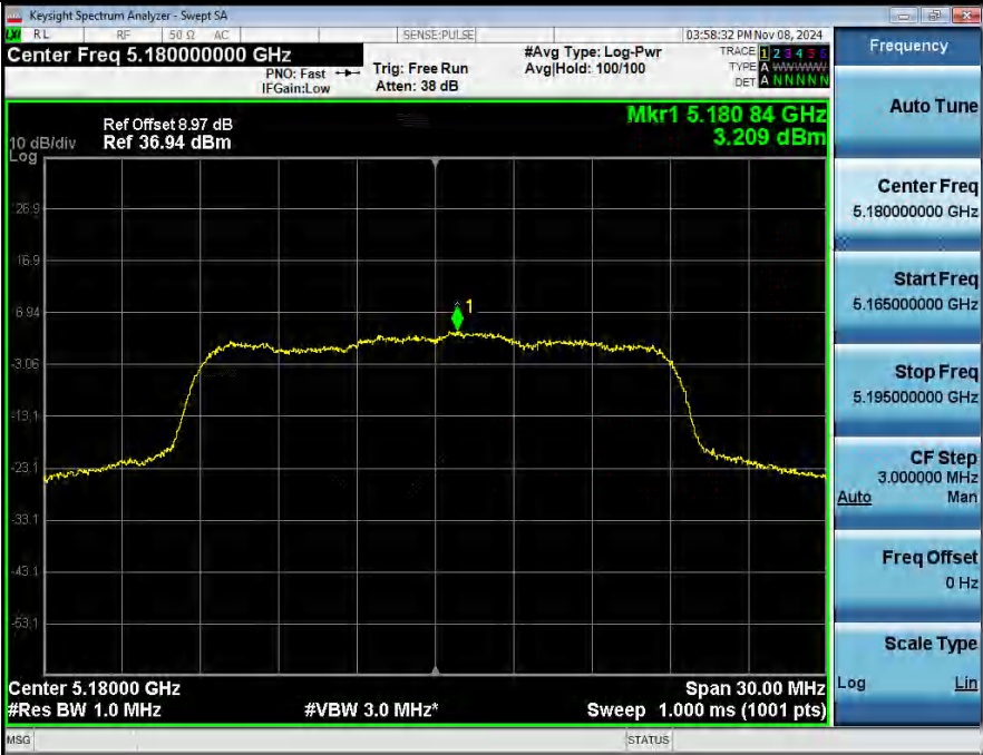
Power Spectral Density NVNT_ANT2_802_11ac(VHT20)_5180
