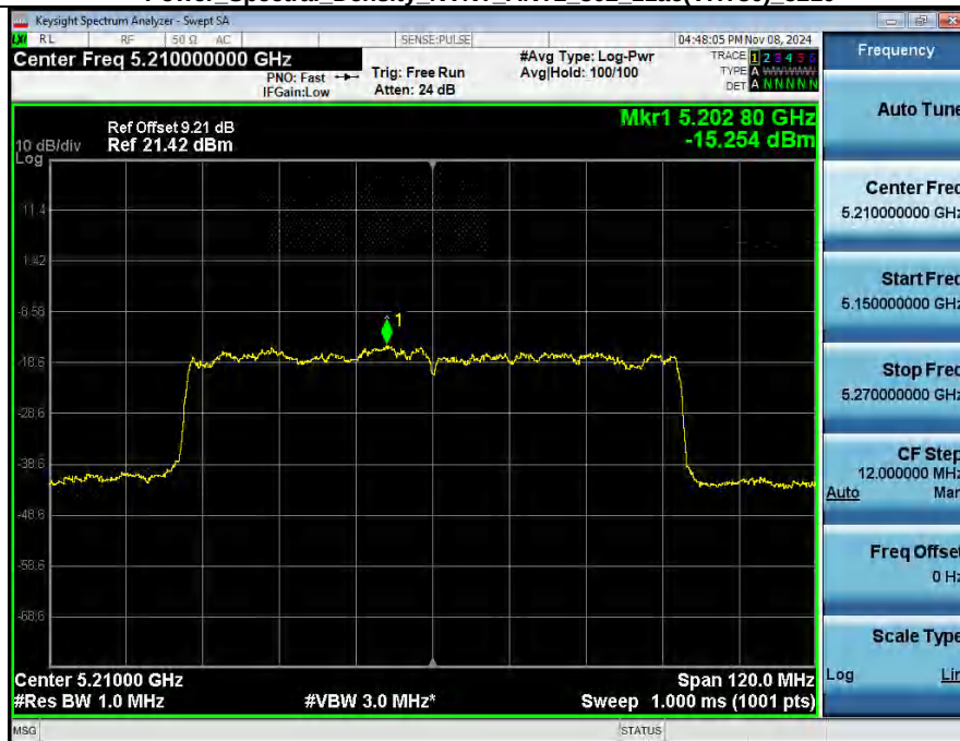
Power Spectral Density NVNT ANT2 802_11ac(VHT80) 5210
