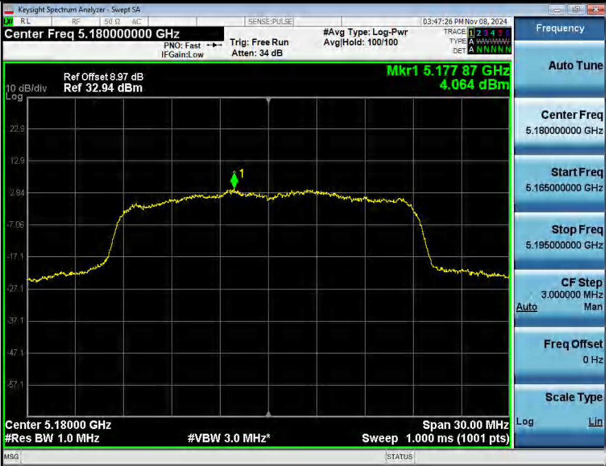
Power Spectral Density NVNT_ANT2_802_11n(HT20)_5180
