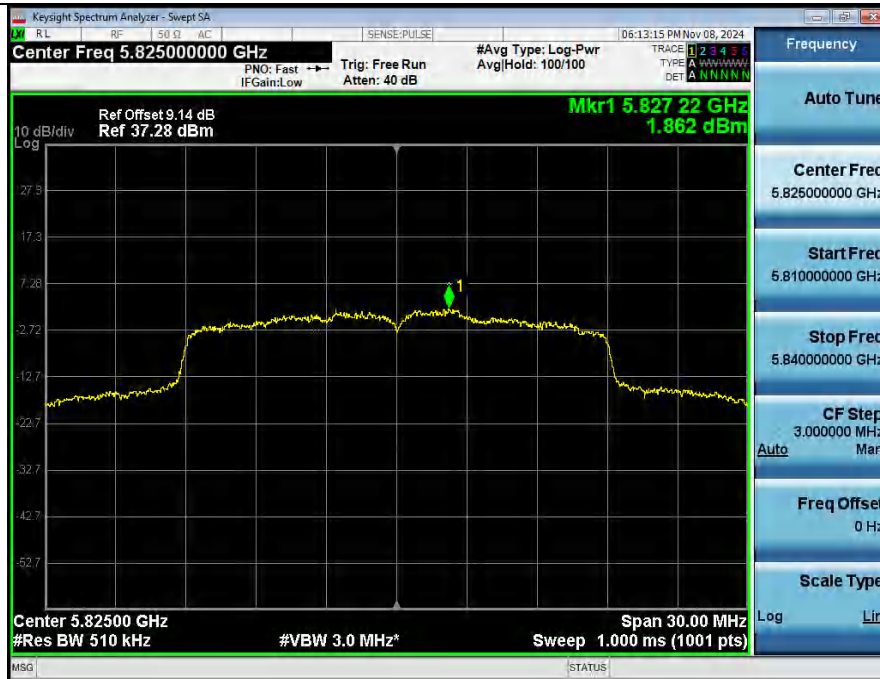
Power Spectral Density NVNT ANT2 802_11ac(VHT20) 5825
