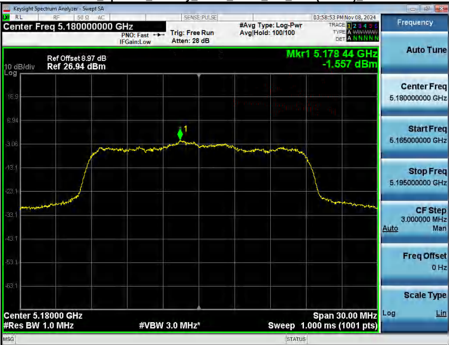
Power Spectral Density NVNT_ANT2_802_11ac(VHT20)_5180
