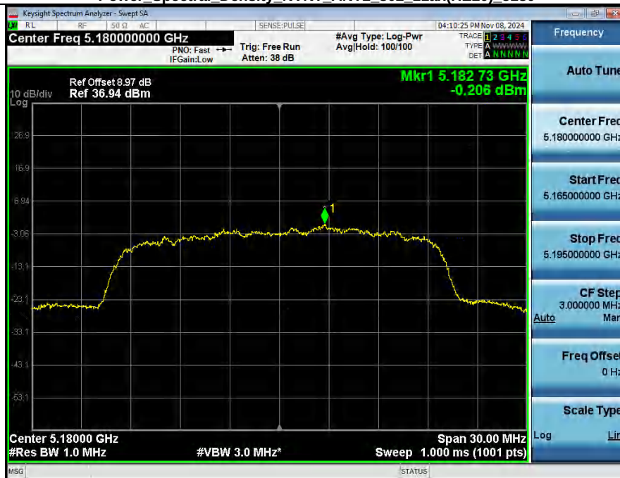
Power Spectral Density NVNT ANT2 802_11ax(HE20) 5180
