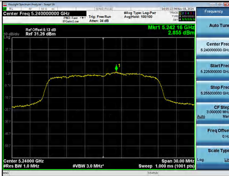
Power Spectral Density NVNT ANT2_802_11ac(VHT20)_5240
