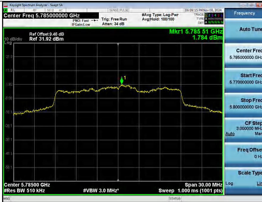
Power Spectral Density NVNT_ANT2_802_11ac(VHT20)_5785
