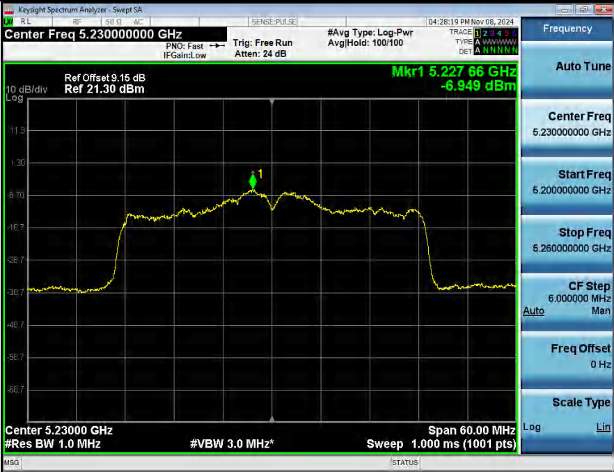
Power Spectral Density NVNT_ANT2_802_11n(HT40)_5230
