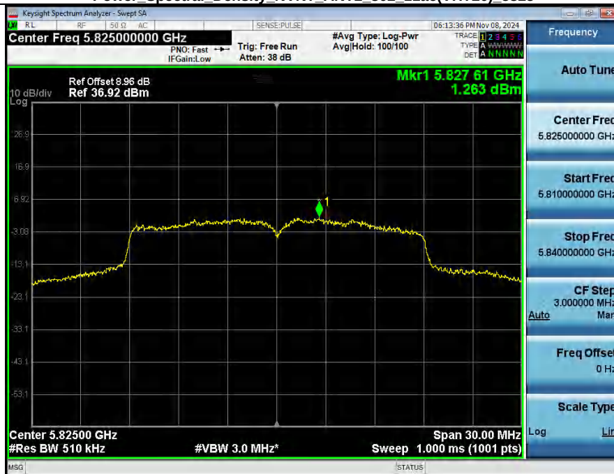
Power Spectral Density NVNT ANT2 802_11ac(VHT20) 5825
