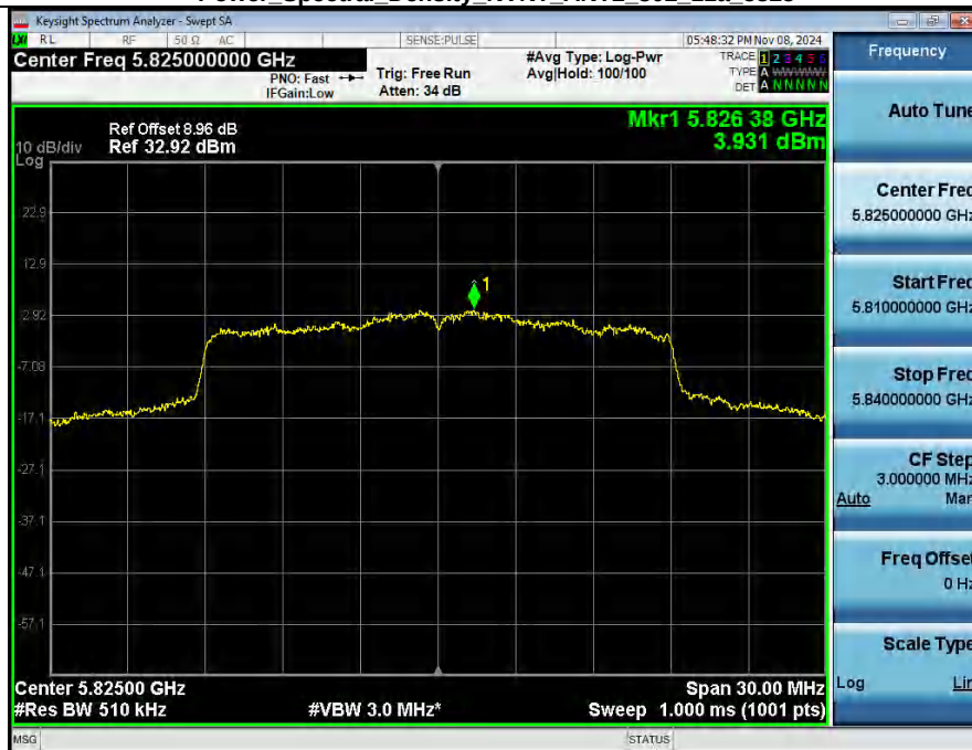
Power Spectral Density NVNT_ANT2_802_11a_5825
