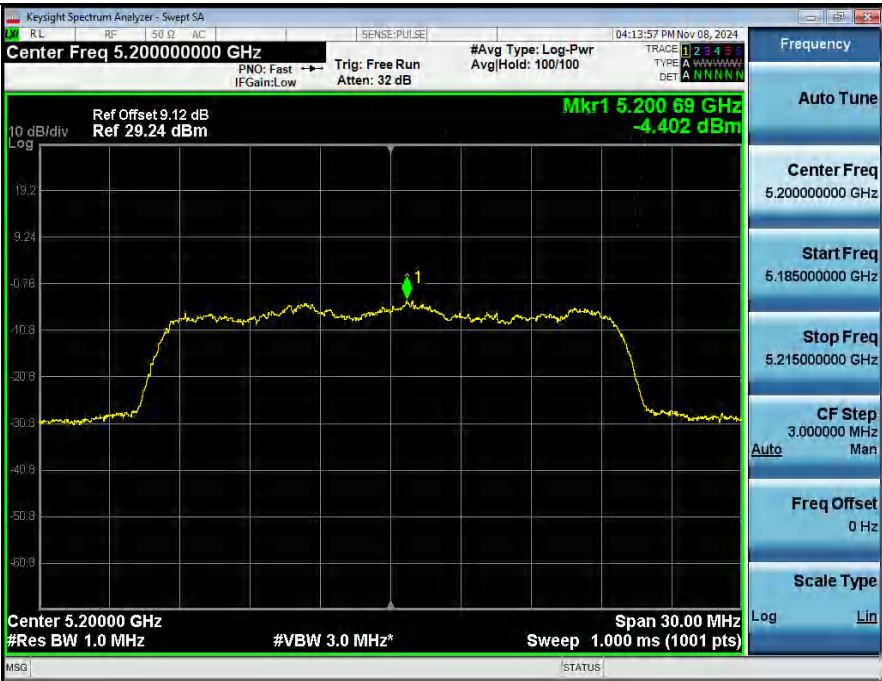
Power Spectral Density NVNT ANT2 802 11ax(HE20) 5200
