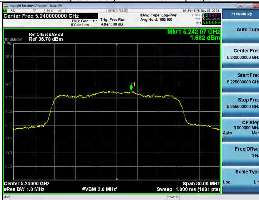
Power Spectral Density NVNT_ANT2_802_11n(HT20)_5240
