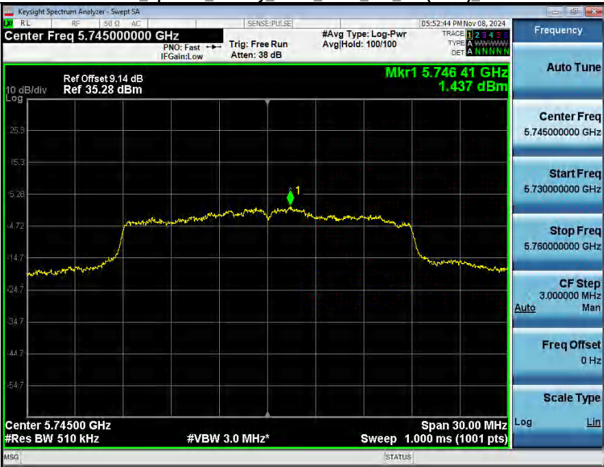
Power Spectral Density NVNT ANT2 802 11n(HT20) 5745
