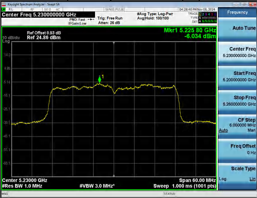
Power Spectral Density NVNT_ANT2_802_11n(HT40)_5230
