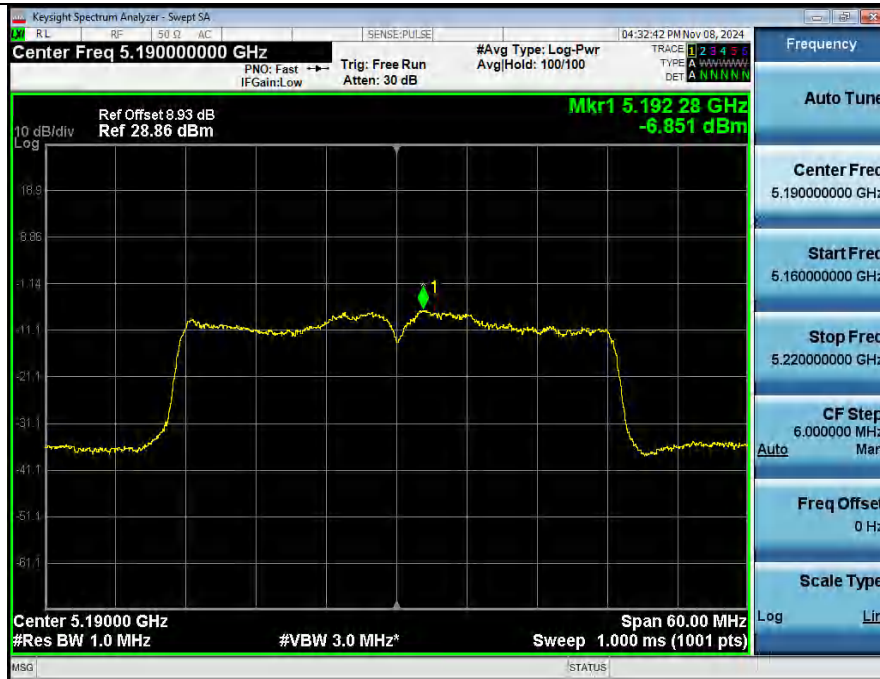
Power Spectral Density NVNT_ANT2_802_11ac(VHT40)_5190
