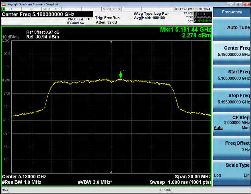
Power Spectral Density NVNT_ANT2_802_11n(HT20)_5180
