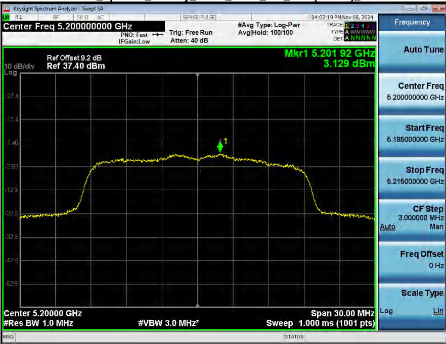
Power Spectral Density NVNT_ANT2_802_11ac(VHT20)_5200
