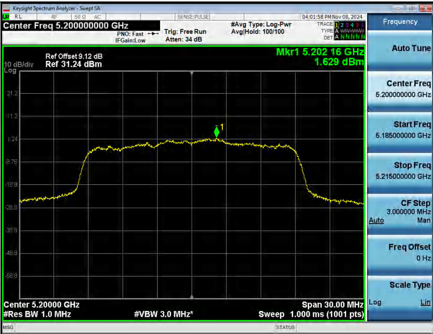
Power Spectral Density NVNT_ANT2_802_11ac(VHT20)_5200
