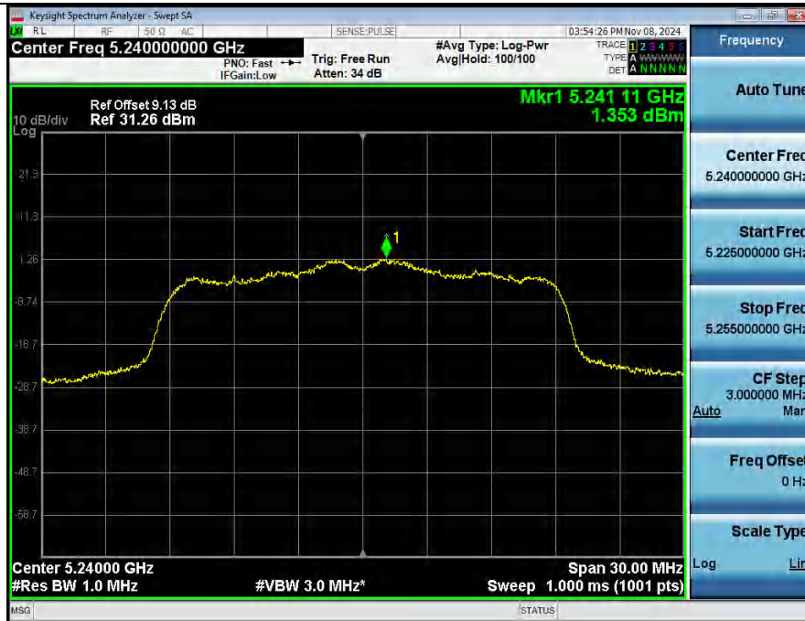
Power Spectral Density NVNT_ANT2_802_11n(HT20)_5240
