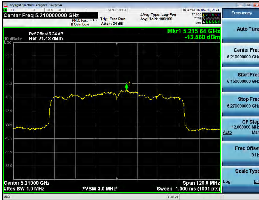
Power Spectral Density NVNT ANT2 802_11ac(VHT80) 5210
