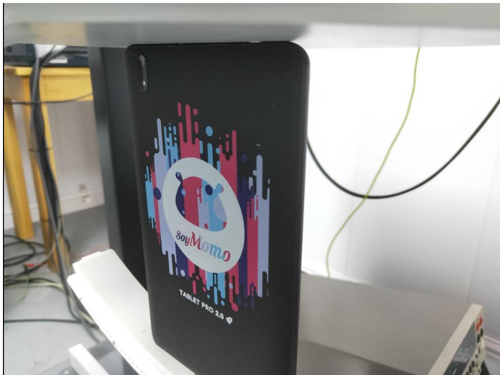
0mm body-worn Left Side Setup Photo
