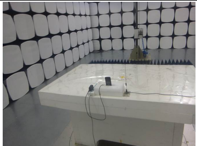
Radiated Spurious Emissions Test Setup Above 1GHz
