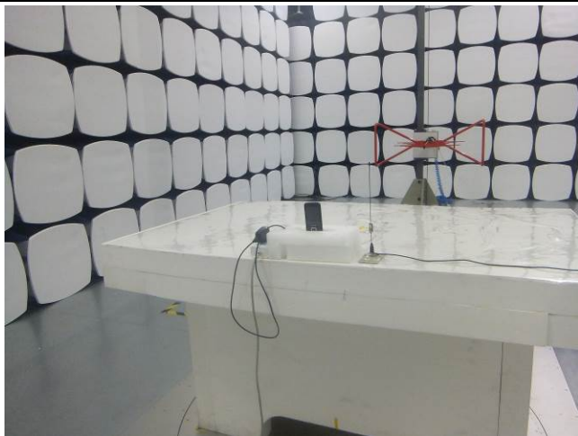
Radiated Spurious Emissions Test Setup Below 1GHz
