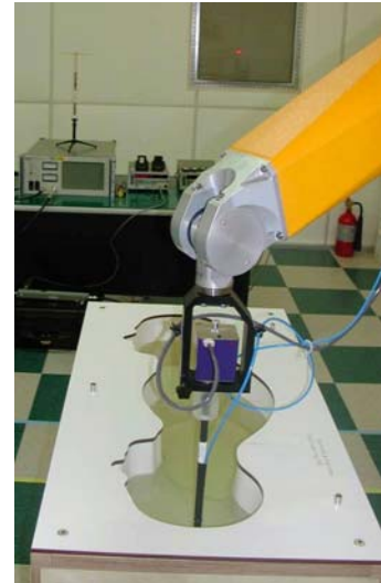
Figure 4. Photograph of the probe and the Phantom
