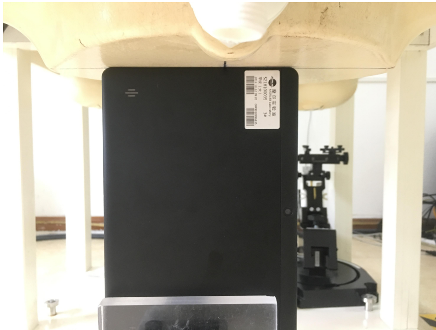
Body worn _ Right (Test distance: 0mm, Thickness of DUT: 10mm)
