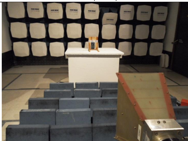
Radiated Emissions (>1GHz) – Front View
