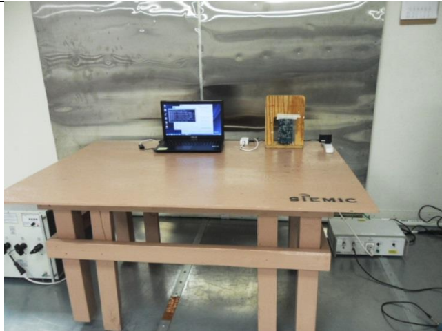
AC Line Conducted Emissions – Front View
