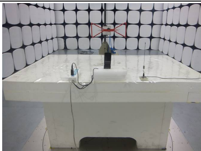
Radiated Spurious Emissions Test Setup Below 1GHz
