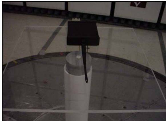
Close-up view of EUT, showing the EUT antenna orientations during testing Vertical orientation Horizontal orientation
