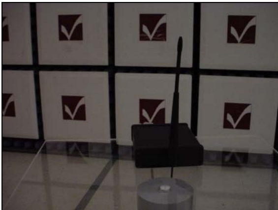
Close-up view of EUT, showing the EUT antenna orientations during testing Vertical orientation Horizontal orientation
