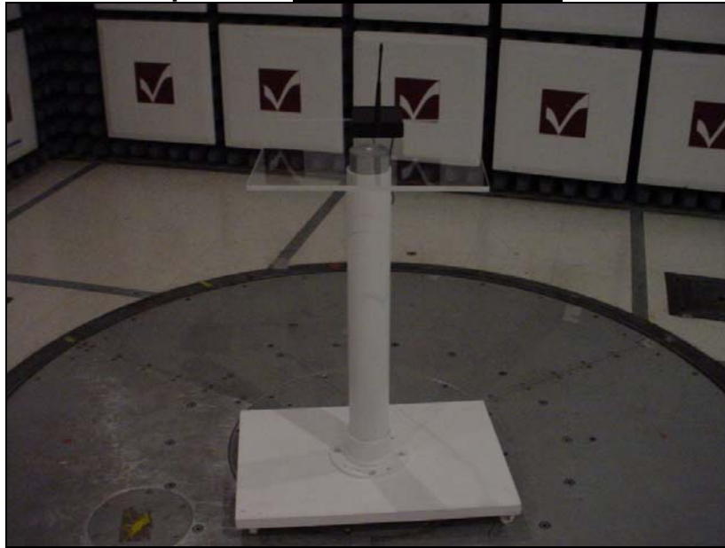
Setup for the Radiated Emissions Test
