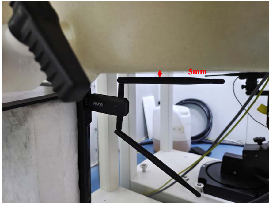
Vertical-Back Adding USB extension cable Setup Photo (5mm)
