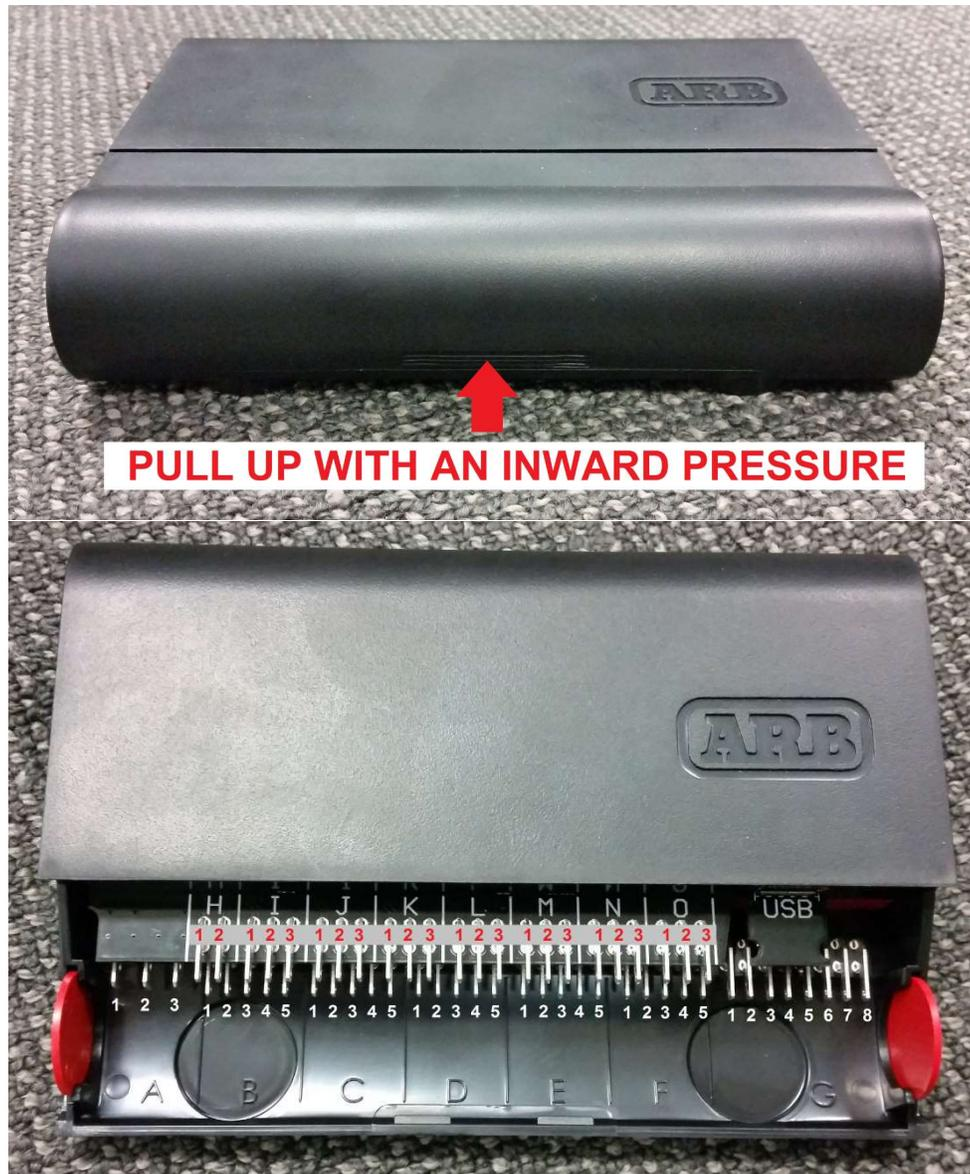
2. Connect the controller to 12V DC power by attaching the positive lead to terminal A1, and the negative terminal to A2.
