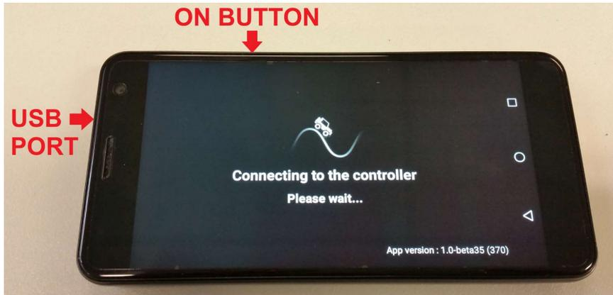
4. Switch on the display by long-pressing on the ON BUTTON as above. The display may take a few minutes to boot up.
