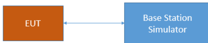
Test Setup FCC Part 22/24/27/90 Cellular; Frequency stability
