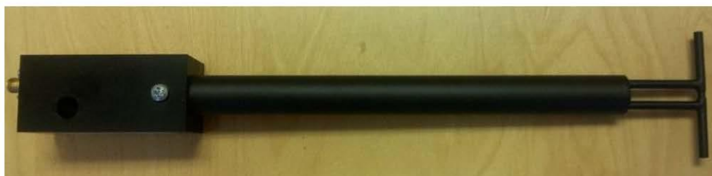
Figure 1 – MVG COMOSAR Validation Dipole
