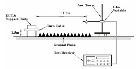
The radiated emission tests were performed in the 3 meters chamber test site, using the setup accordance with the ANSI C63.10-2013. The specification used was the FCC 15.209, FCC 15.407 limits.
