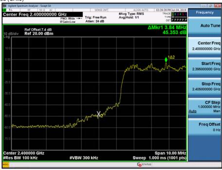
Test Plots with hopping ( $\pi/4DQPSK$ )
