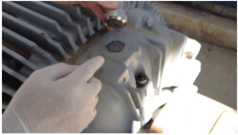
Note: It is important that the Mote is mounted with the Petasense logo facing the direction of the machine's shaft for orientation purposes
