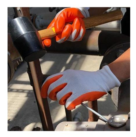
Step 3: Clean the Mount by chipping away any leftover epoxy residue with the Chisel/Rubber Hammer. A Handheld Grinder can also be used to clean the Mount.
