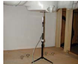
Figure 11.1 Dipole Verification Test Setup Diagram & Photo
