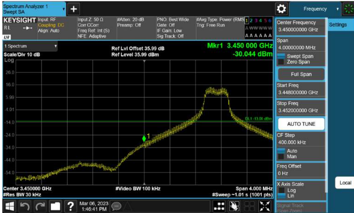
Sub6 n77(78). Low Band Edge Plot (80 M BW Ch.632668 BPSK 1RB)(1)
