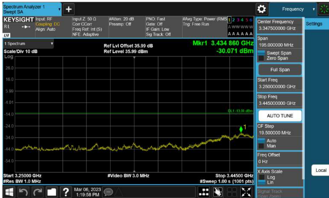
Sub6 n77(78). Low Band Edge Plot (60 M BW Ch.632000 BPSK FullRB)(3)
