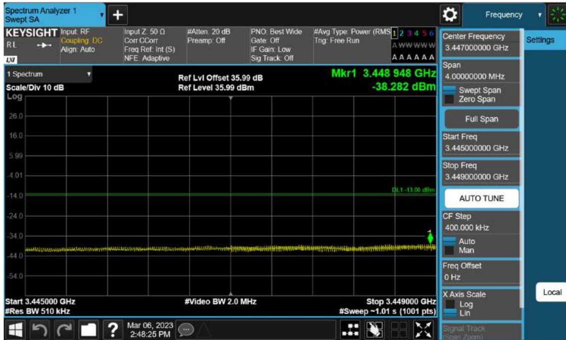
Sub6 n77(78). Low Band Edge Plot (100 M BW Ch.633334 BPSK FullIRB)(2)
