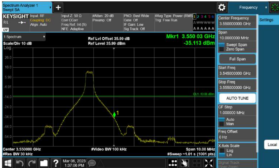
Sub6 n77(78). High Band Edge Plot (70 M BW Ch.634332 BPSK 1RB)(1)
