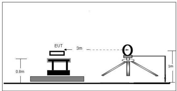
(B) Radiated Emission Test-Up Frequency 30MHz~1GHz
