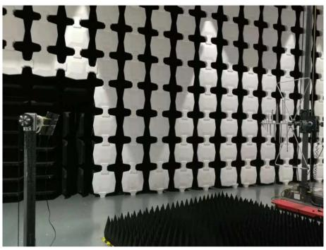
Description: Substitution Antenna for ERP Test
