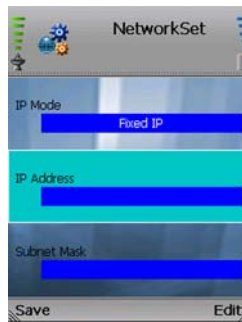
Figure 4-18: Network Settings - Fixed IP
