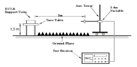
The radiated emission below 1GHz tests were performed in the 3 meters chamber test site A, above 1GHz tests were performed in the 3 meters chamber test site B, using the setup accordance with the ANSI C63.10-2013. The specification used was the FCC 15.209, and FCC 15.247 limits and the RSS-247 Clause 5.5, RSS-GEN Clause 8.10 limits.
