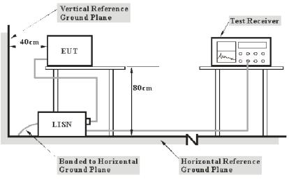
Note: 1. Support units were connected to second LISN. 2. Both of LISNs (AMN) 80 cm from EUT and at the least 80 cm from other units and other metal planes support units.
