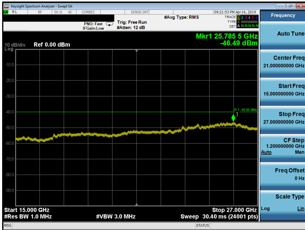
Plot 7-83. Conducted Spurious Plot (Band 30 - 10.0MHz QPSK - RB Size 1, RB Offset 0 - Mid Channel)
