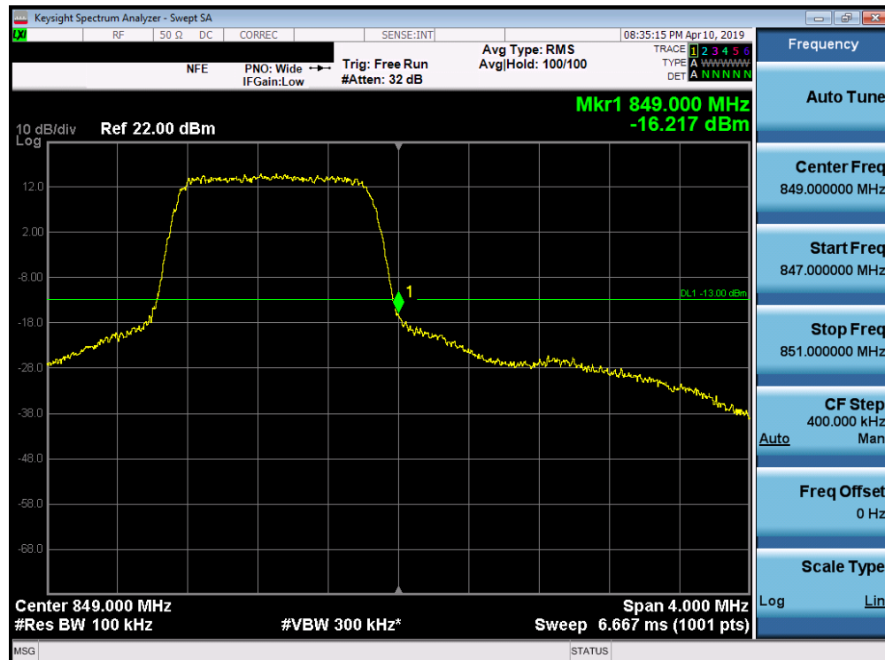
Plot 7-93. Upper Band Edge Plot (Band 5 - 1.4MHz QPSK - Full RB Configuration)
