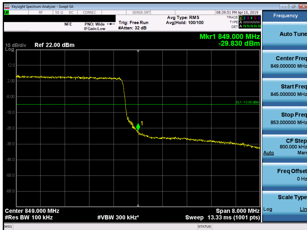
Plot 7-99. Upper Band Edge Plot (Band 5 - 10.0MHz QPSK - Full RB Configuration)
