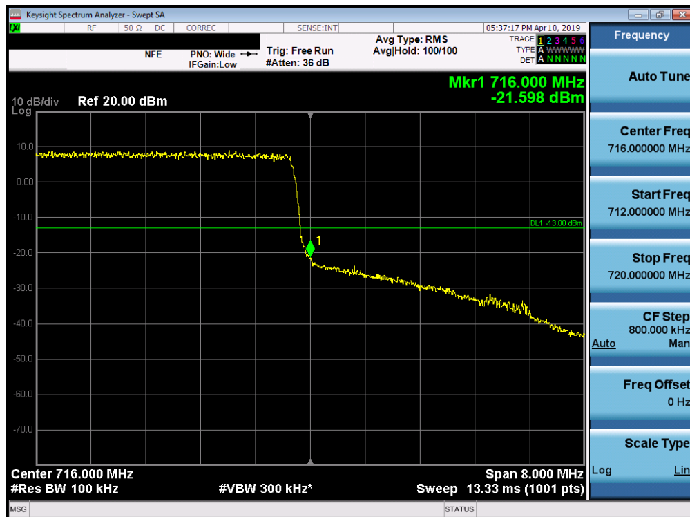
Plot 7-89. Upper Band Edge Plot (Band 12 - 5.0MHz QPSK - Full RB Configuration)
