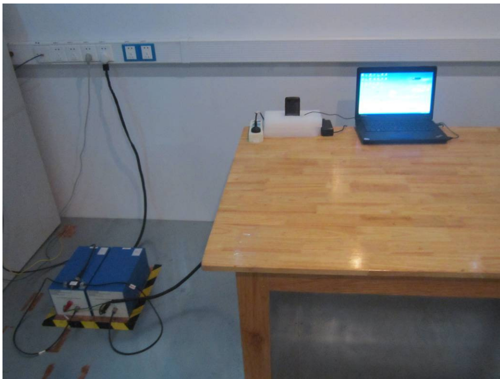
Conducted Emissions Test Setup Front View
