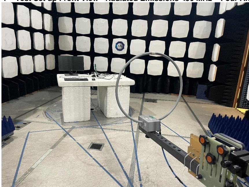
Figure 2 – Test Set up Front View - Radiated Emissions <30 MHz – Two Antennas
