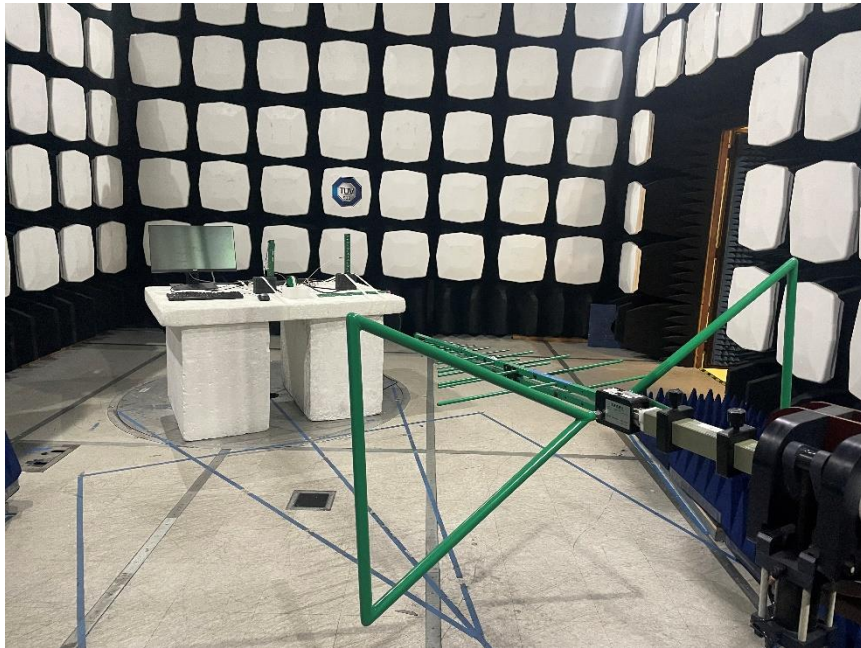
Figure 5 – Test Set up Front View - Radiated Emissions <1 GHz – Four Antennas
