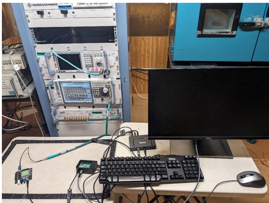
Figure 14 – Test Set up – Antenna Port Measurement
