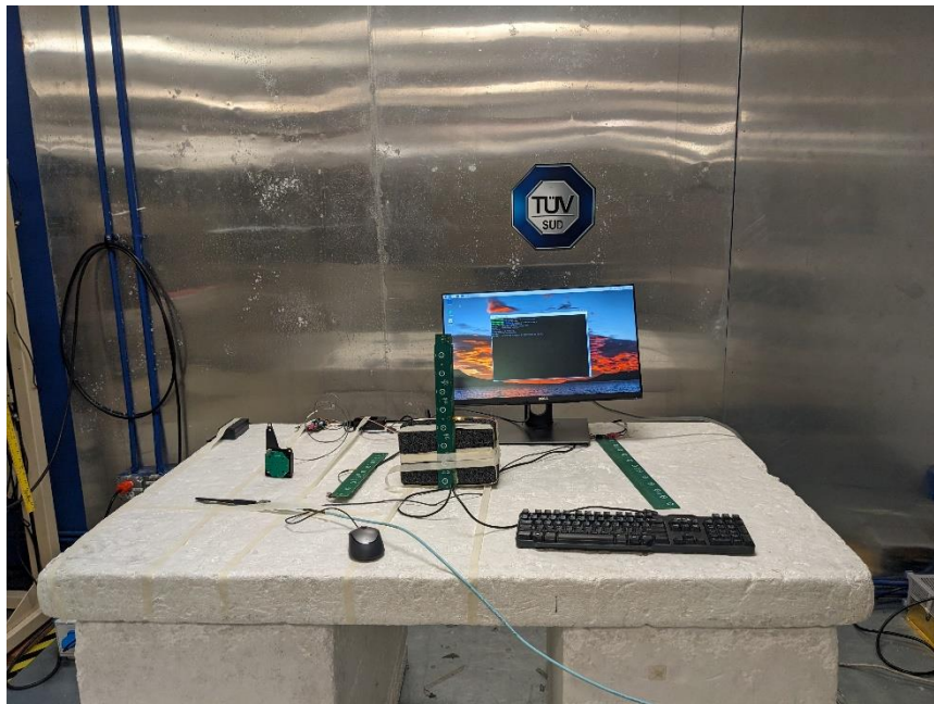
Figure 13 – Test Set up – Conducted Emissions
