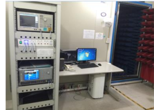
Pegatron's SATIMO SG24 chamber
