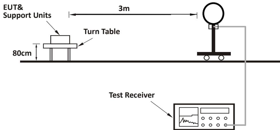
For Radiated emission 30MHz to 1GHz:
