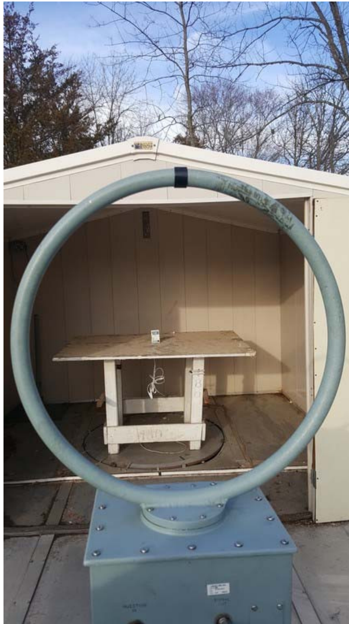
Figure 3.3 Radiated Configuration Test Setup
