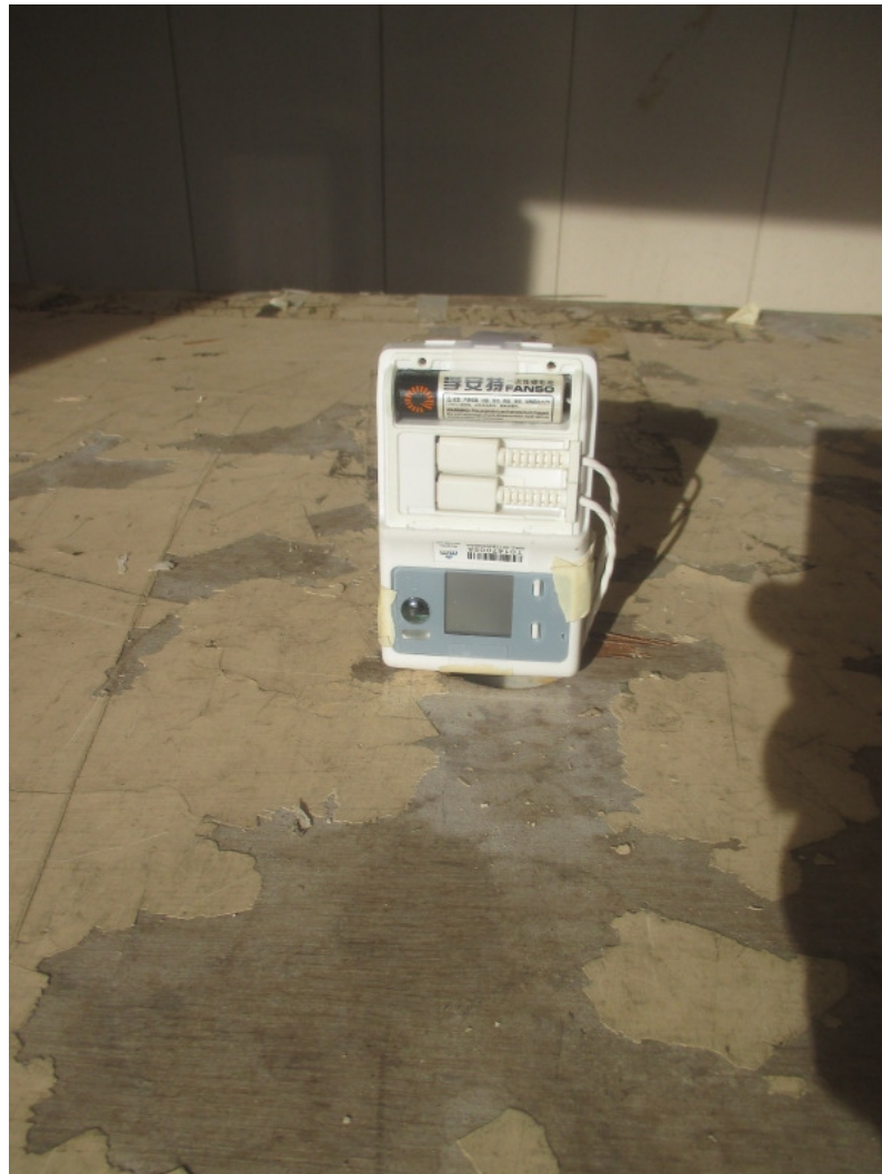
Figure 3.2 Radiated Test Setup position 2 (Button Down)
