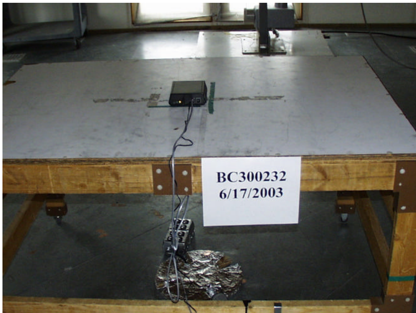
Test-setup photo(s): Radiated Emissions
