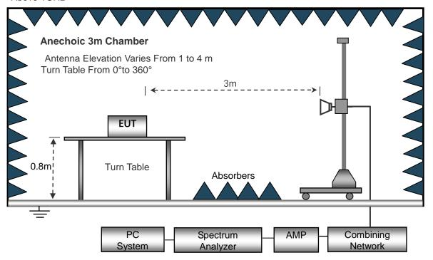
6.2 Test Standard and Limit FCC PART 15 B Below 1GHz
