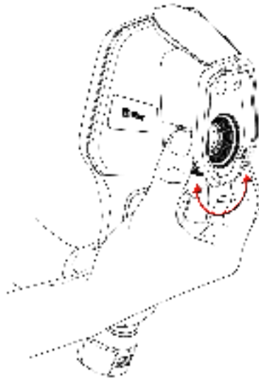
Figure 8.1 Focus Adjustment Through Focus Ring
