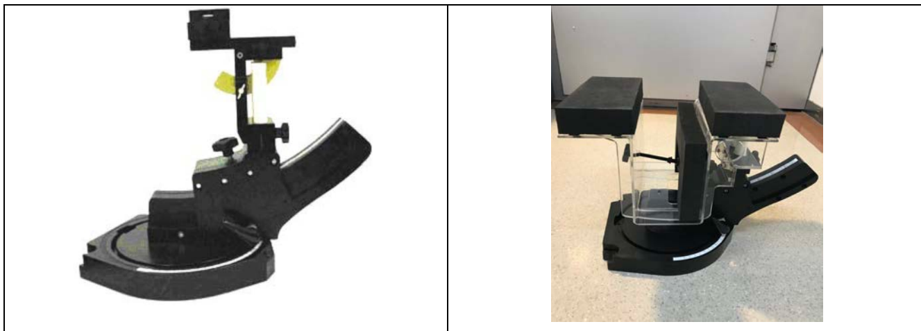
Device holder supplied by SPEAG
