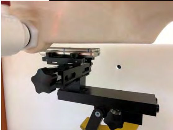
Fig.7 EUT Front side to flat phantom
