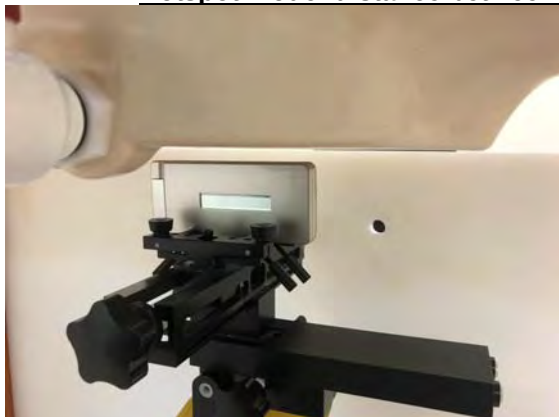
Fig.13 EUT Right side to flat phantom
