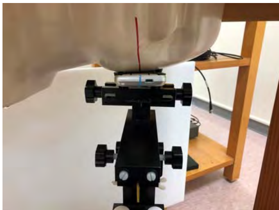
Fig.5 Left Head Section / Cheek-Touch Position
