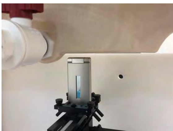
Fig.12 EUT Top side to flat phantom
