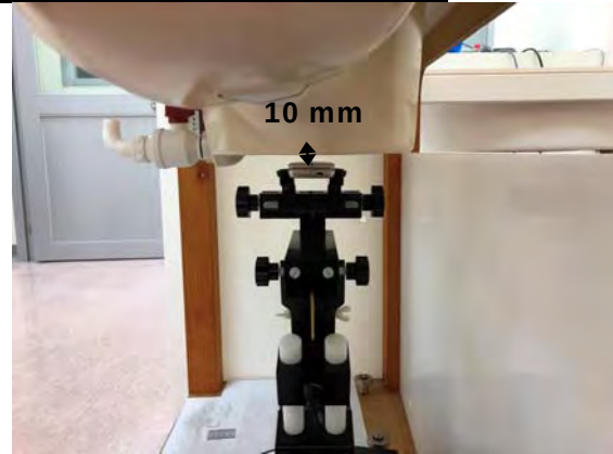
Fig.7 EUT Front side to flat phantom
