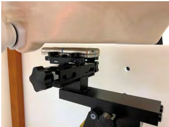
Fig.8 EUT Back side to flat phantom
