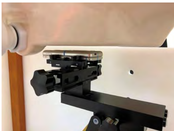
Fig.11 EUT Back side to flat phantom
