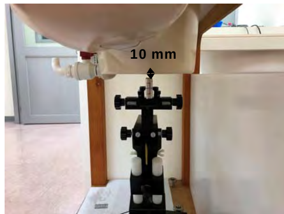
Fig.14 EUT Left side to flat phantom
