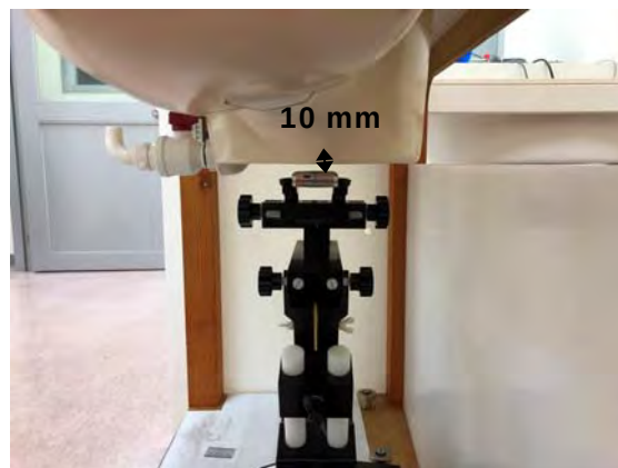
Fig.11 EUT Back side to flat phantom
