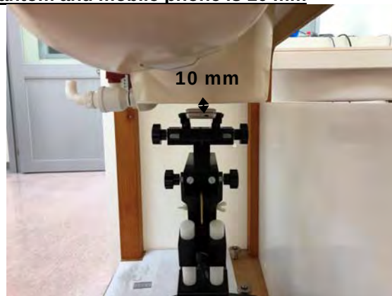
Fig.10 EUT Front side to flat phantom
