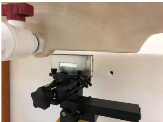
Fig.14 EUT Left side to flat phantom
