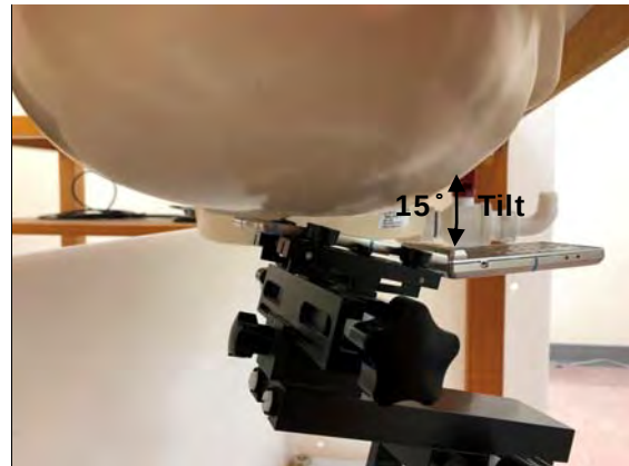
Fig.4 Right Head Section / Ear-Tilt Position(15°)
