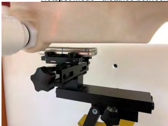
Fig.10 EUT Front side to flat phantom
