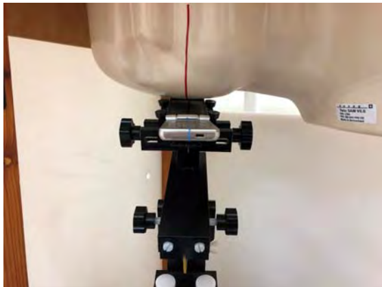
Fig.4 Right Head Section / Ear-Tilt Position(15°)
