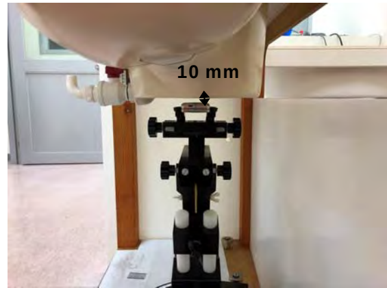
Fig.8 EUT Back side to flat phantom
