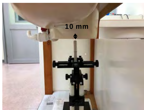
Fig.12 EUT Top side to flat phantom
