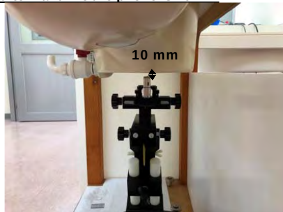
Fig.13 EUT Right side to flat phantom
