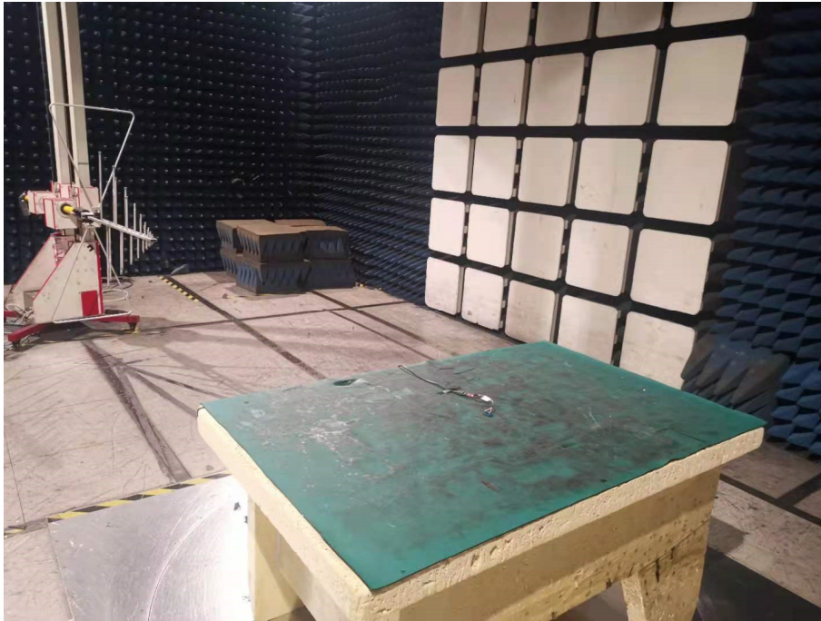
Spurious Emission Test Setup (Below 1GHz)
