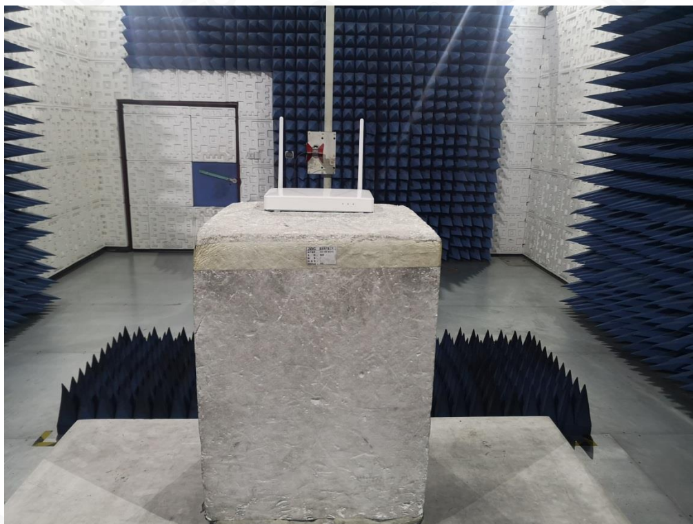
FCC RADIATED EMISSION TEST SETUP ABOVE 1GHZ
