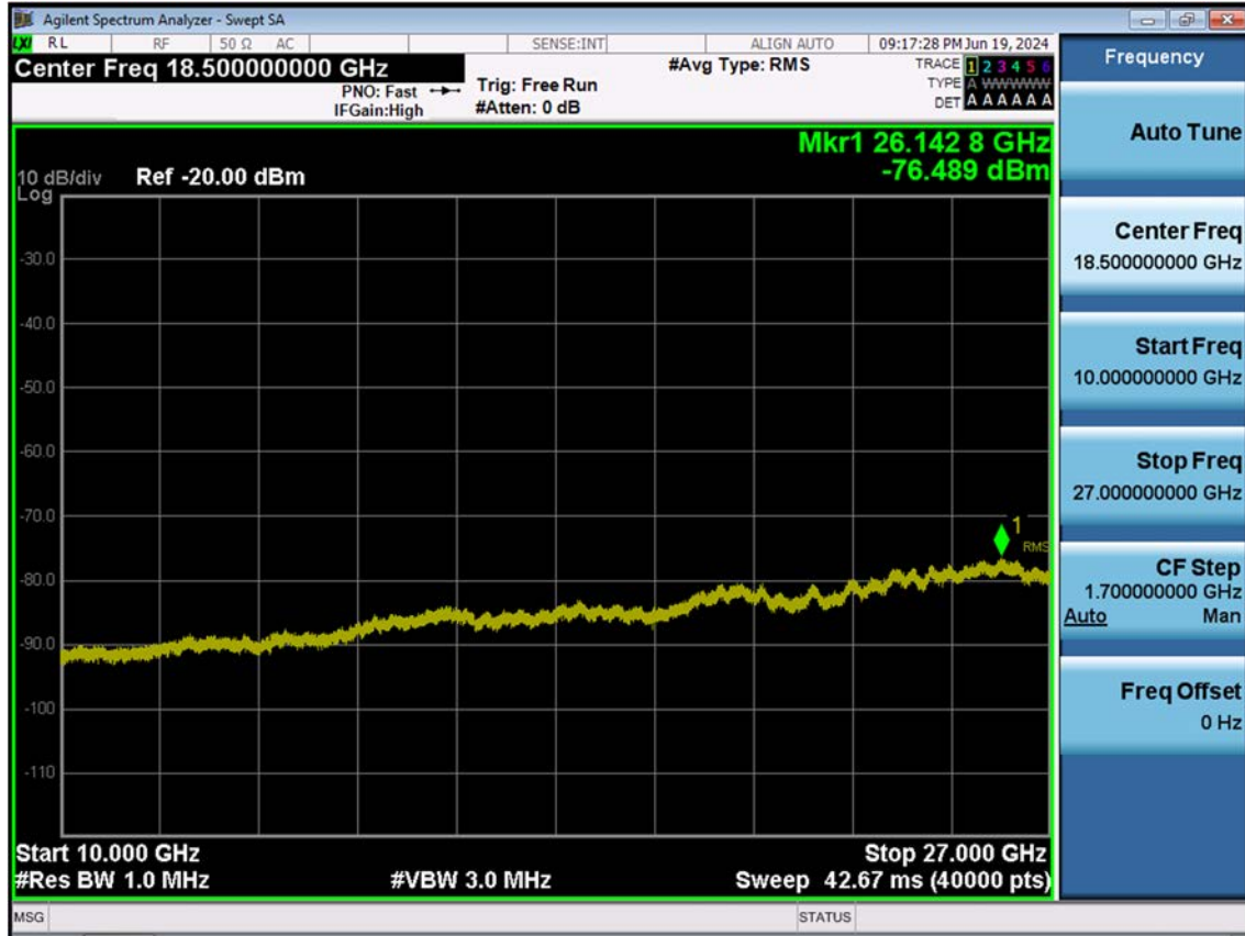
LTE B41_20 M_Conducted Spurious(Above10 G)_Low_QPSK_1RB
