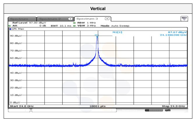
Note: The Average limit of fundamental is 107.96  $dB\mu V/m@3$  m, and the maximum measure Peak level of fundamental is 91.31  $dB\mu V/m@3$  m which is below 107.96  $dB\mu V/m@3$  m, worst case of fundamental is recorded in this report
