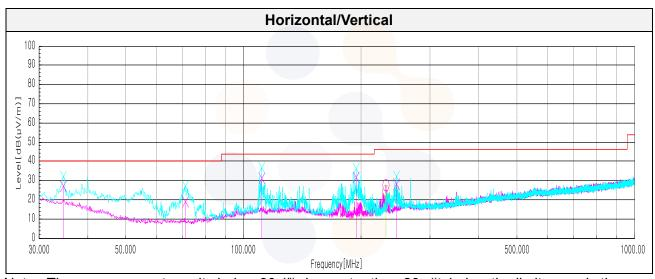
Note : The measurement results below 30  $\, \text{Mb} \,$  is greater than 20  $\, \text{dB} \,$  below the limit, so only the radiated spurious emissions from 30  $\, \text{Mb} \,$  to 100  $\, \text{Gh} \,$  were reported.
