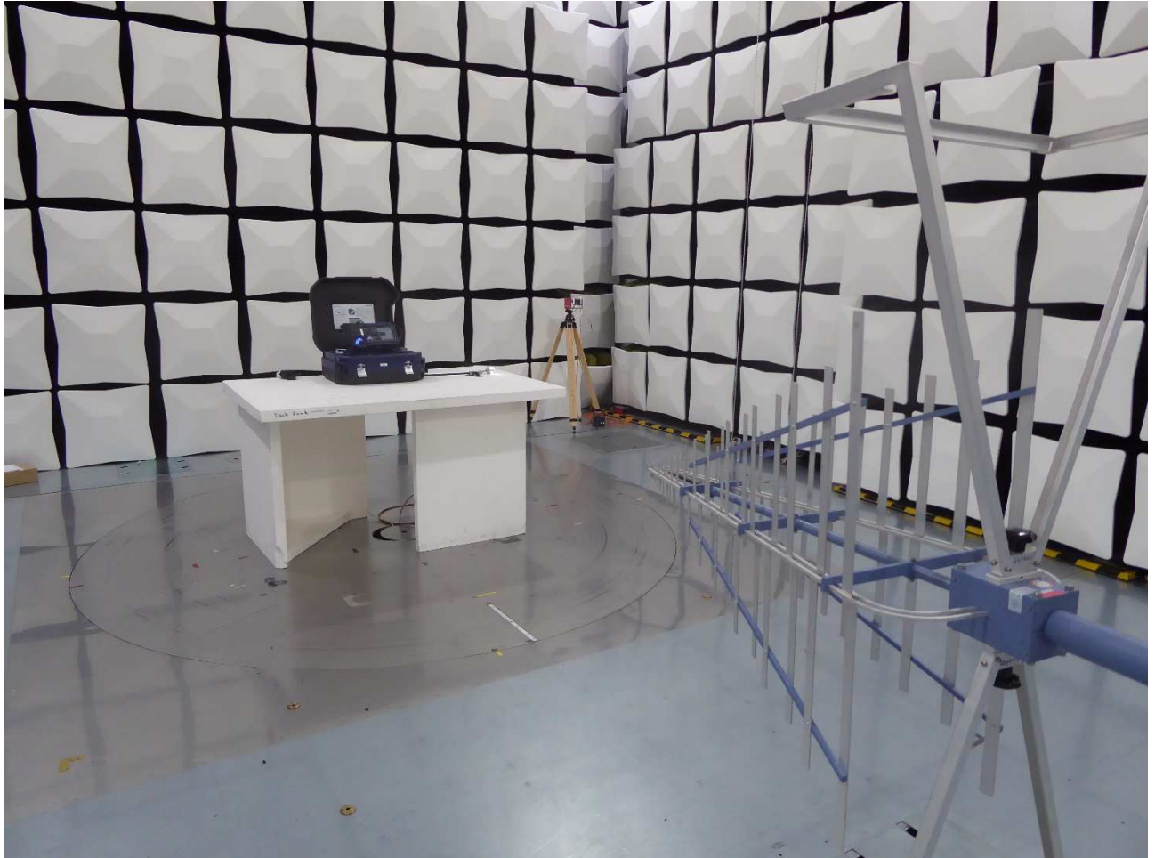
Test setup semi anechoic chamber (30 MHz – 1 GHz)
