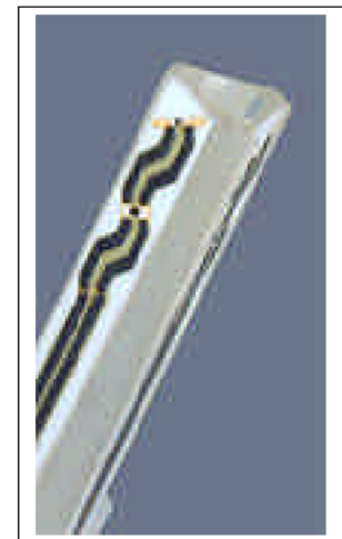
Inside view of ET3DV6 E-field Probe
