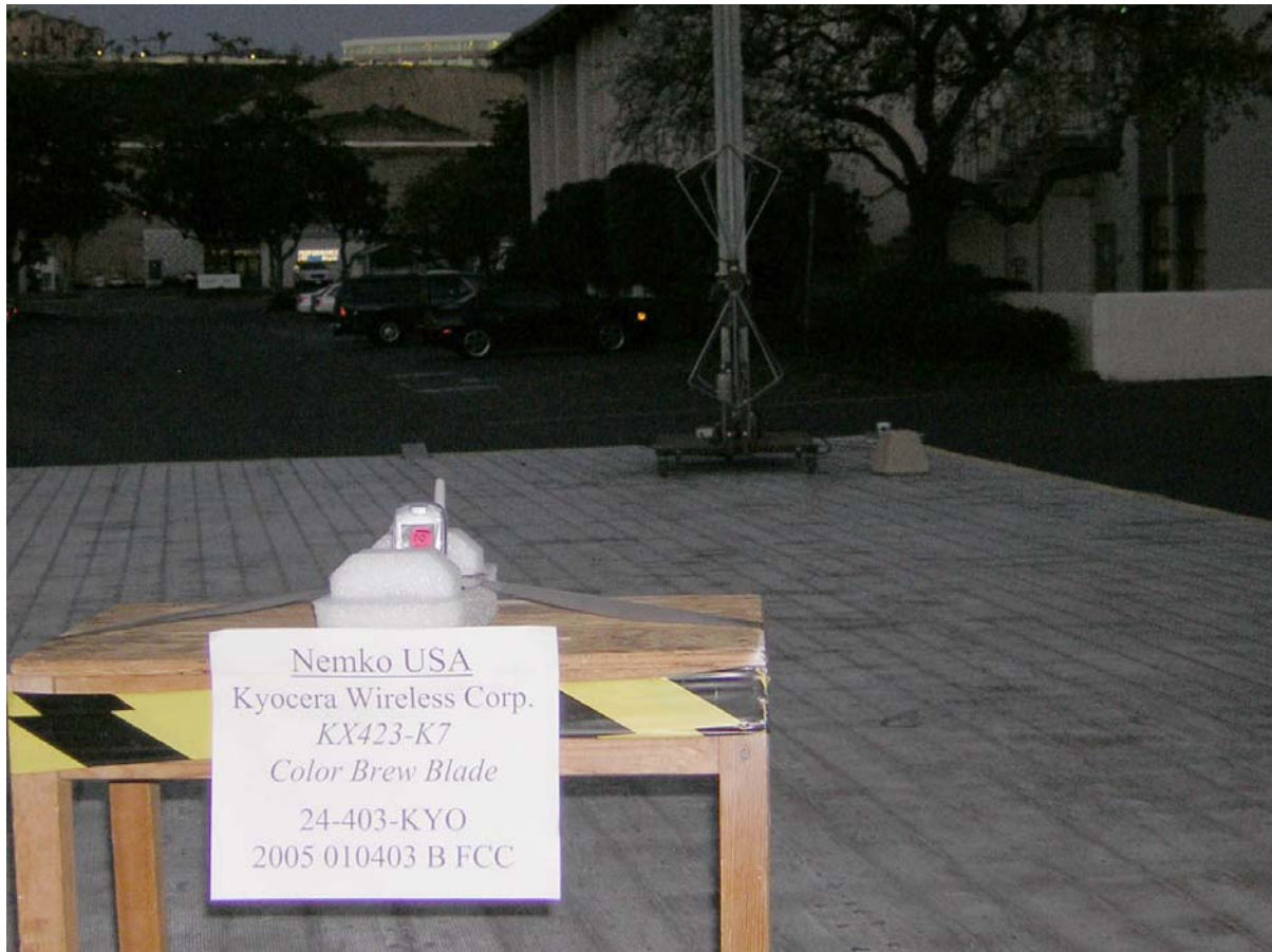
Photograph 2. FCC, Part 15 Radiated Emissions Test Configuration
