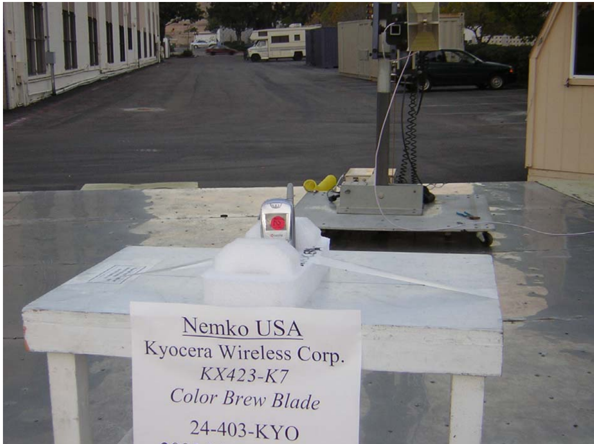
Photograph 1. FCC, Part 24 Radiated Emissions Test Configuration
