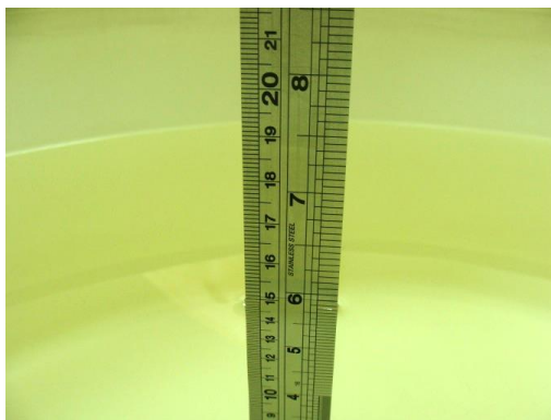
Fig 6.1 Photo of Liquid Height for Body SAR
