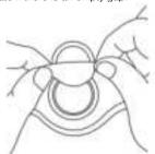
**6** Arrange the microphone module with the KOROT sensor cover as shown below, and cover it with the case that was removed at the beginning.
