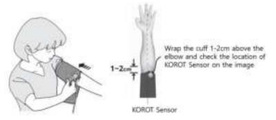
• After locating the KOROT sensor on the proper position, wrap the cuff and tighten it by using the Velcro.
