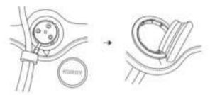
• Hold the band of the old KOROT sensor cover and remove it.
