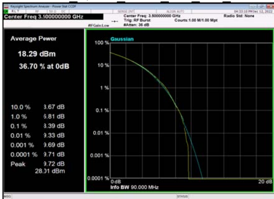
N77(90M)_CP-OFDM QPSK Outer Full Mid CH
