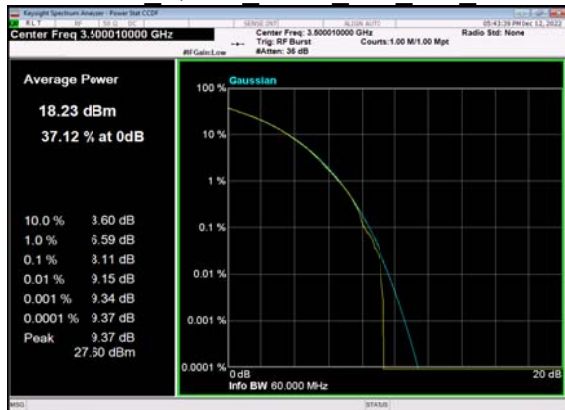
N77(60M)_CP-OFDM QPSK Outer Full Mid CH
