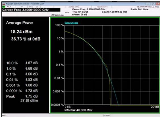
N77(40M)_CP-OFDM QPSK Outer Full Mid CH
