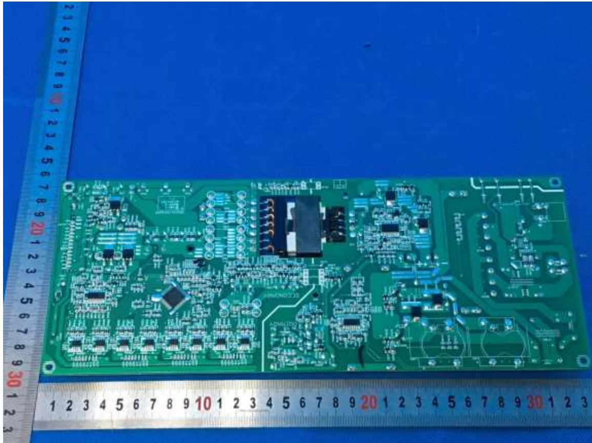
Picture 16 – Power board view (Model FSP194-2FS01)
