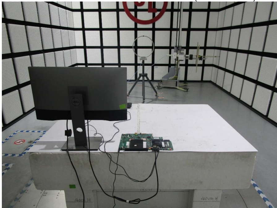
RADIATED RF MEASUREMENT SETUP (Below 30MHz)
