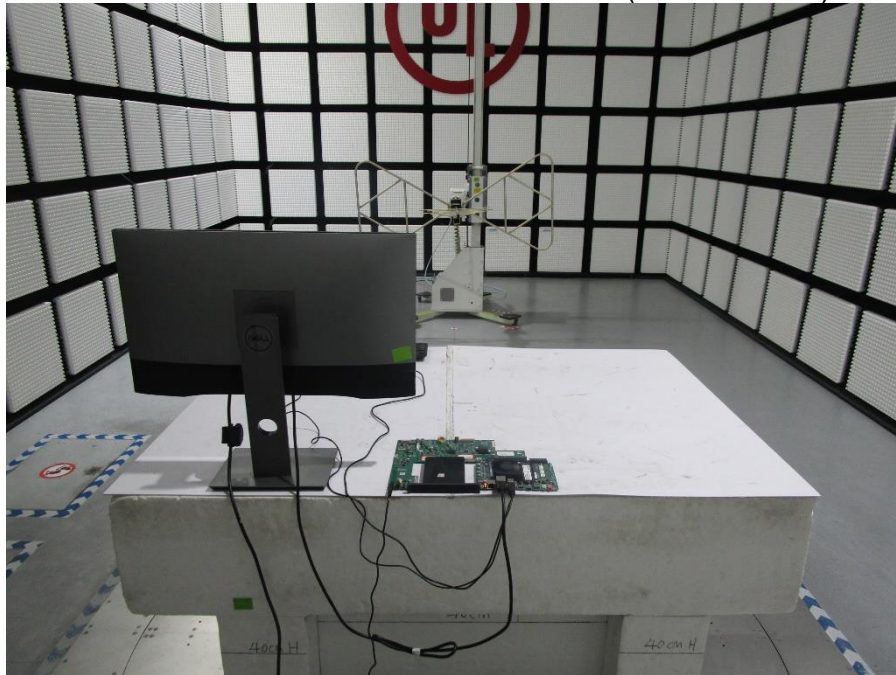
RADIATED RF MEASUREMENT SETUP (Below 30MHz)
